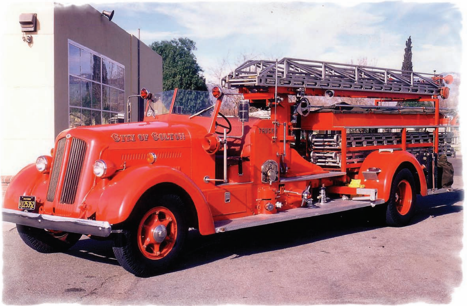
1942 Seagraves 50' Aerial Ladder Truck that remained in service till 1982. This was an easy test for fear of heights. Not because of the height but once you were at the tip of the ladder, it would move around like a loose branch. Just the slightest wind or when the water came rushing to the top and would charge the monitor tip pushing 500 to a 1000 gallons a minute - you better hang on because you are in for a ride. This unit was originally a pumper and the men took the 50' aerial from an earlier modified International pickup.
